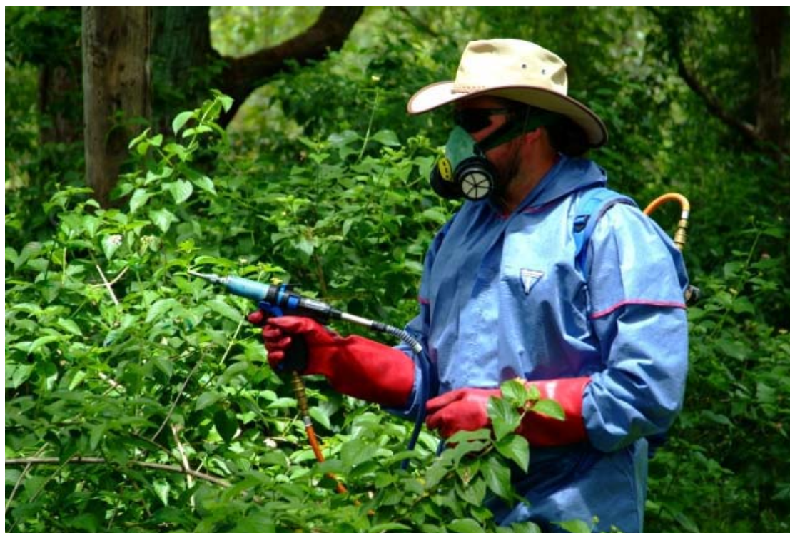
Fig 4. The NJ Phillips Forestry Gas Gun has been specifically developed for the delivery of a stream of herbicide over extended distances.
